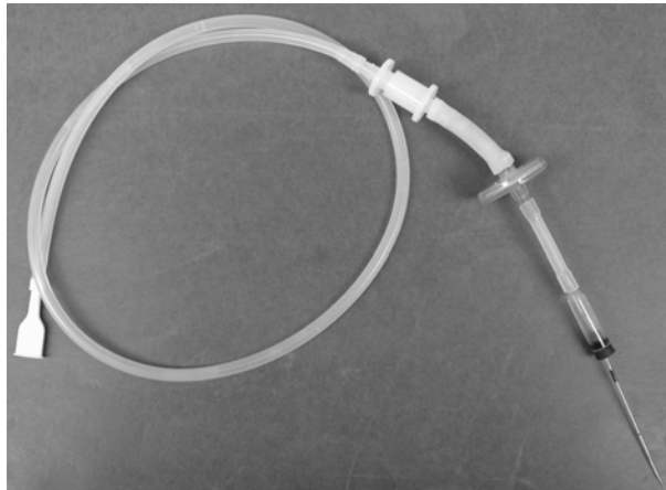
Figure 2.1. Apparatus used for cell isolation. A drawn out capillary pipette (lower right) attached to one end of a piece of silicon tubing and a mouthpiece is attached to the other.
